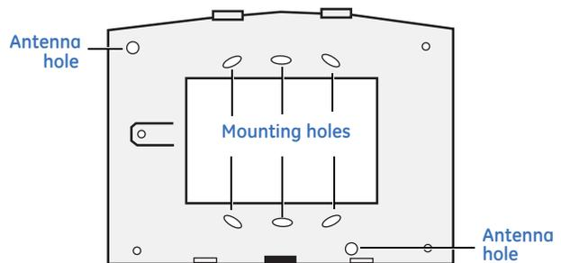
3. Drill 15/64 in. holes at the marked antenna hole locations.
